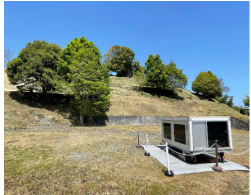
Fig. 3 Measurement device installed at location P1. The device was placed horizontally, oriented toward the central axis of the mound in the posterior circle.
