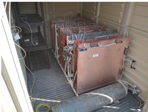
Fig. 3 A photograph of the muographic observation system with its gas system and power supply system.
