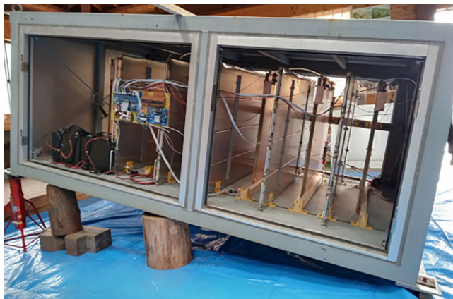
Figure 3. Photograph of the muographic observation instrument that was assembled from six gaseous tracking detectors and five 2-cm-thick lead plates (Oláh et al. 2018).
